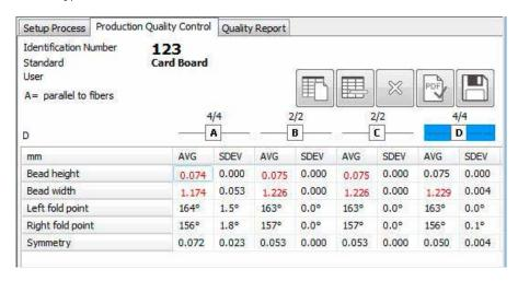
Out-of-tolerance values are highlighted in red.
