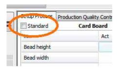
Once a reference for a card board material or a box blank is available it is still necessary to setup the embosser before starting production. In this case check the Standard selector to compare actual readings with reference numbers. If the current readings are out of tolerance, the numbers will be displayed in red.
